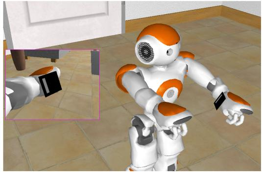
Fig. 1. Illustration of the robotic setup. A marker is placed on the hand of the robot providing visual feedback of its end-effector position.
