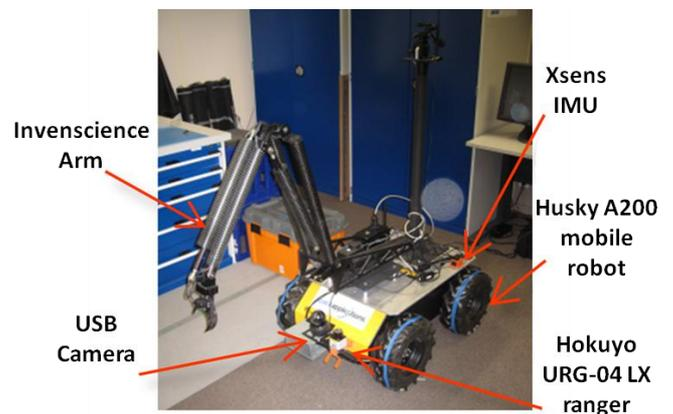
Figure 1. Outdoor mobile manipulator platform
