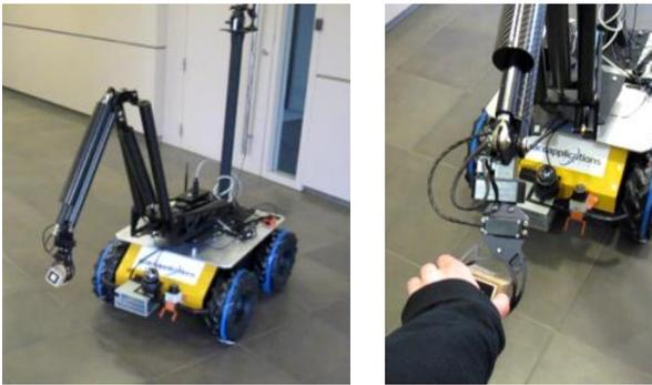
Figure 3. Motor babbling learning (left) and grasping action execution (right)
