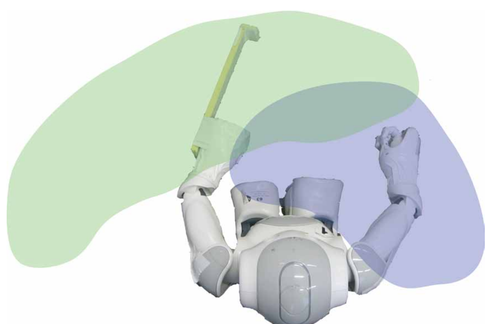
Figure 2. Top-down view of the Nao with an illustration of the reachable space for each end-effector.
