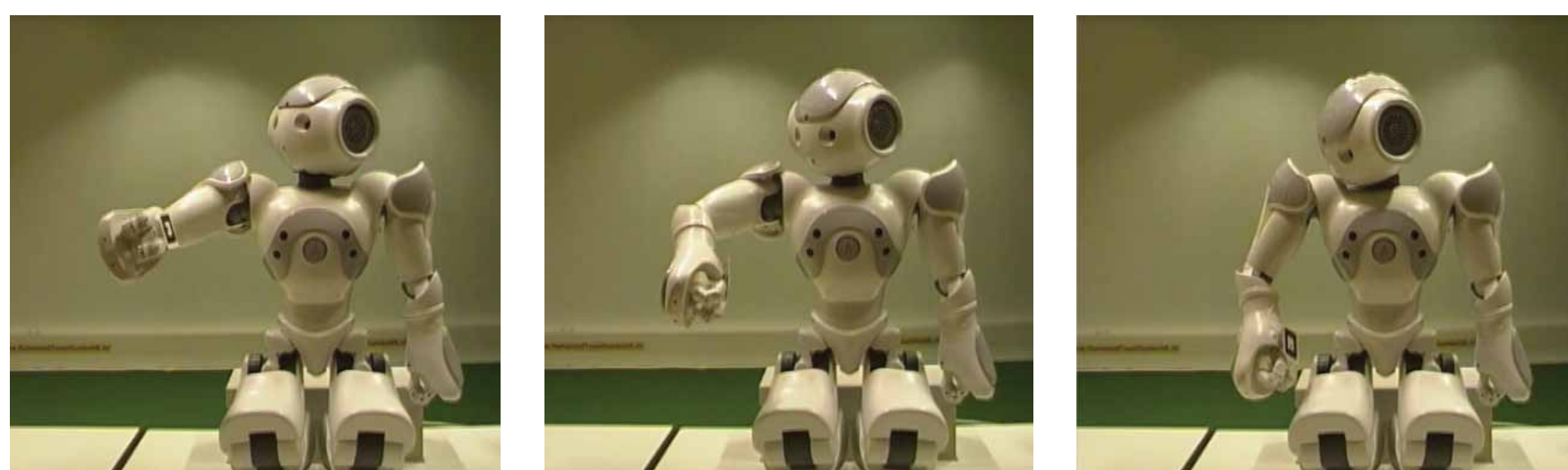
Figure 1. Body Babbling for learning the sensorimotor schemes that code for the capabilities of the arms
